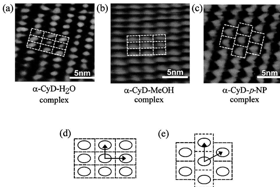
Fig. 3. STM images of (a)  $\alpha$ -CyD-H<sub>2</sub>O, (b)  $\alpha$ -CyD-MeOH, and (c)  $\alpha$ -CyD-*p*-NP inclusion complexes and their structural models with (d) twofold and (e) threefold symmetric arrangement.
